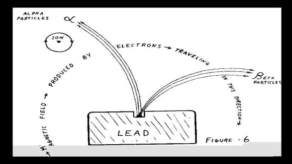
Here we have a piece of radium inside of the hollow depression in the lead block as shown. . Around this we have a strong magnetic field.
