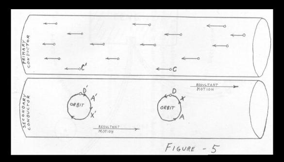
Ordinarily at frequencies such as commercial power frequencies of sixty cycles per second, these wires will be wound around a soft iron core and at frequencies of hundreds of thousands of cycles per second and millions of cycles per second a ferrite core can be used to obtain a maximum transfer of power from the primary (top conductor in our Figure 5.) to the secondary (bottom conductor in the same figure).
